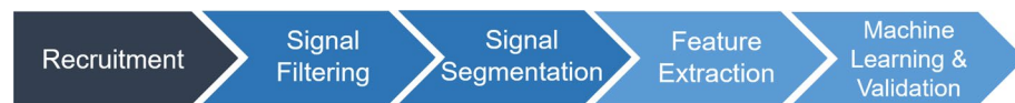
Figure 6. The experimental process of this study. After the fNIRS signal is obtained, it will be filtered, segmented and extracted and imported to machine learning to get classification results, and finally confirm the credibility of the results with cross-validation.
